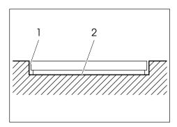
Always keep gap (1) between weighing platform and base frame free from dirt.
